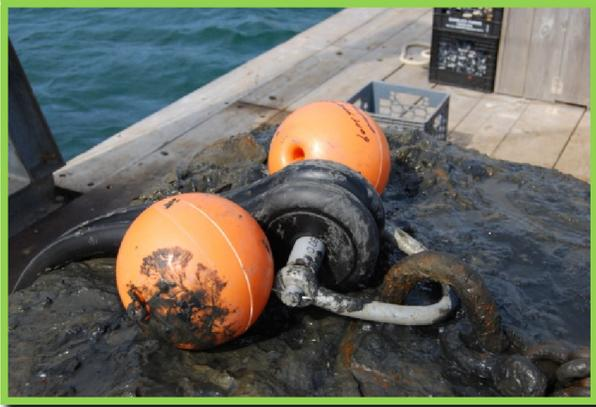
*Photo left: The Hazelett Marine conservation mooring system is attached to the anchor block and is ready to be lowered to the bottom. Notice the gooey black and brown sludge on top of the anchor block. Traditional mooring chains must raise a potent cloud of this silt when they drag across the sea bottom.*
