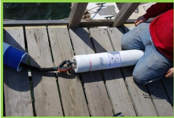
Photo left: The pennant has been secured to the S/S swivel, and James is ready to install the spar buoy cap that will protect the finish of the boat from hardware scratches. The cap also has identification numbers attached to it.
